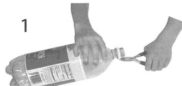
Use a pair of snippers or a nail clipper to remove the retaining ring from the mouth of the bottle. If you don't remove it, the retaining ring can interfere with the positioning of the fins.
